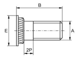
For plate thickness, min = 1.5Head diameter E = 8
